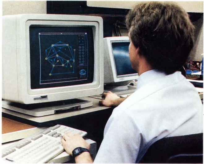
Graphic development tools for Ada programs, such as this directed-graph editor and code generator developed by the Westinghouse Electronic Systems Group (Baltimore, MD), drastically reduce the apparent complexity of an embedded design and clarify the various subunits within a program.
