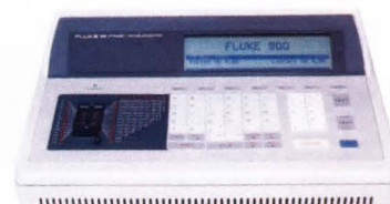
900 Dynamic Troubleshooter tests digital ICs (even proprietary ICs like custom PALs), operating at speed, while still in circuit. Detects static, timing, and intermittent faults.
