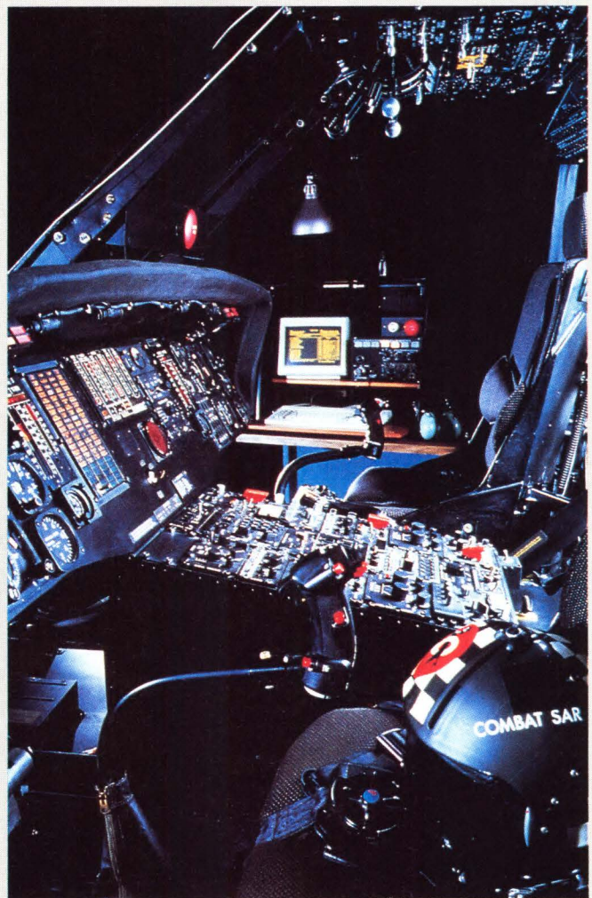
Ada and a personal computer from Zenith operate this UH-60A Black Hawk helicopter trainer for the army. The Ada development system is from Alslys. Many flight simulators and trainers, excellent examples of real-time applications, now incorporate Ada code. (Courtesy Validity Corp)
